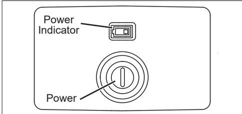
3. Press and hold the Power button to turn off the tool.
