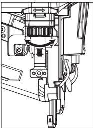
6. Press the workpiece contact bracket against a workpiece 2.
